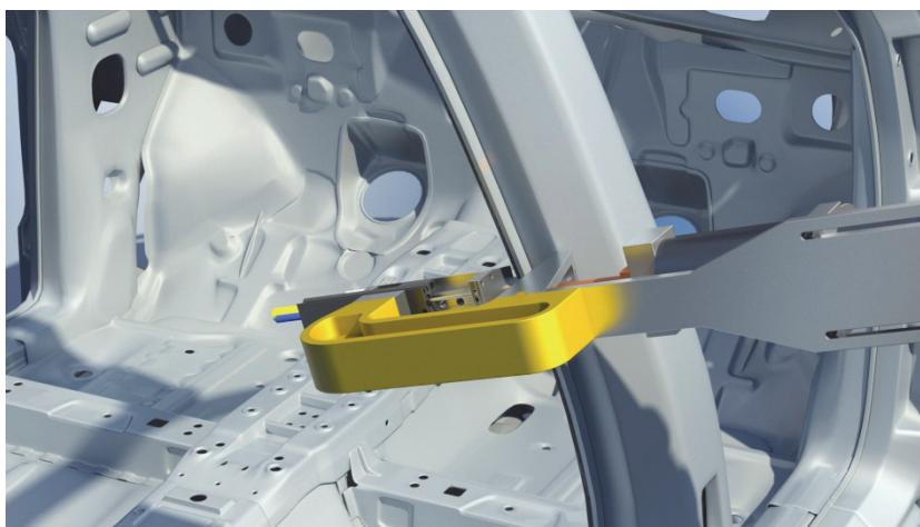
**The HPCI technology is used to integrate composite parts to metallic car body structures.**
